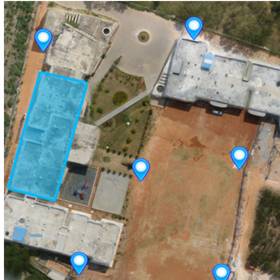
Figure 3: The GCPs are distributed across the building and at the center.
