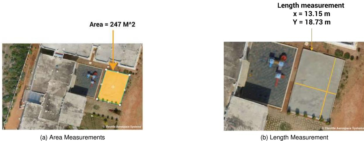
Figure 9: Area and length measurement of the constructed building using TAS UAS
