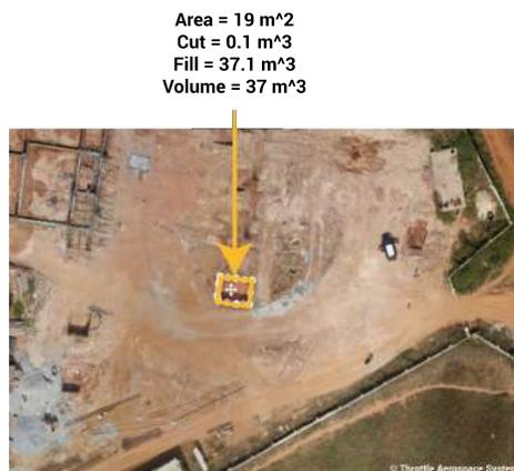
Figure 10: Pit volumetric measurement
