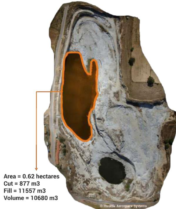
Figure 8: Volume measurements
